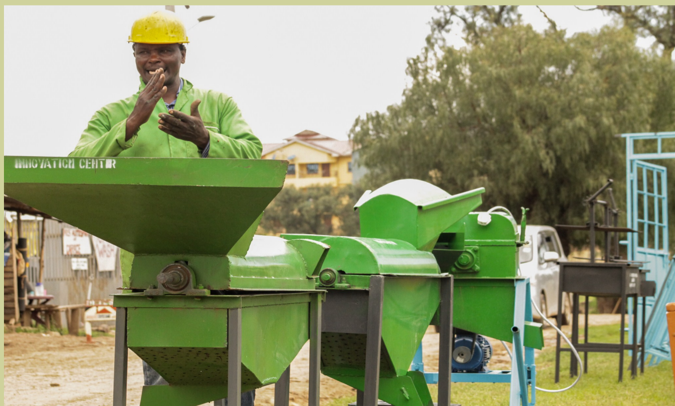
A fuel efficient maize shelling machine manufactured at the centre.
